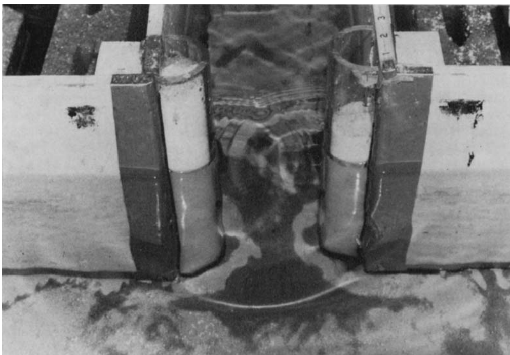
FIGURE 5. Wave-induced sand accumulation near a narrow-mouthed estuary. Waves were normally incident. The wave maker was shut off after the accumulation was established and before photography.
