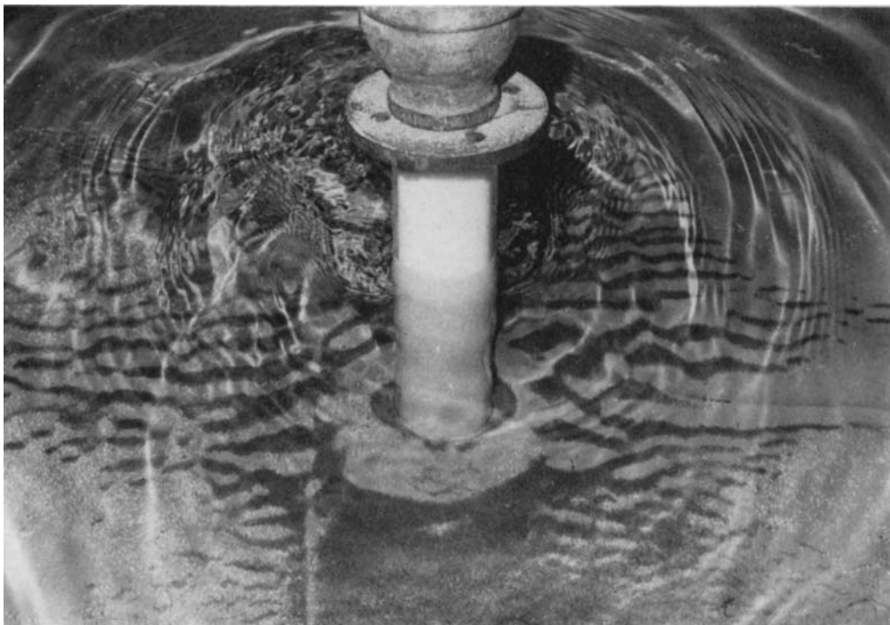
FIGURE 4. Wave-induced sand accumulation near a circular cylinder. Dark spots, stripes and patches indicate sand. The wave crests are parallel to the ripple crests. Sand particles were removed initially from a ring of width 3 cm surrounding the cylinder.
